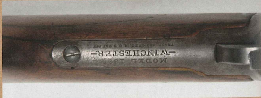
Tang markings on Winchester 1895 Saddle Ring Carbine (SRC). Late-production models bore the inscription "Model 95."
