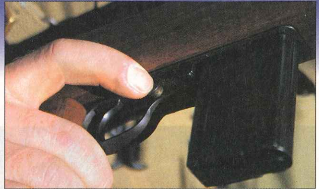
The M1 Carbine's safety was a small button behind the mag release. Because the release was often pressed instead of the safety, the button was later changed to a lever.
