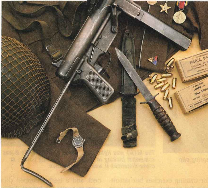
The M3 “Grease Gun” submachine gun was also an issue item. Like the Thompson, it chambered .45 ACP ammo, but it was much cheaper and easier to build than its predecessor. Many parts were stamped and welded. The M3 combat knife was a popular item. It was later adapted for use as a bayonet on the M1 Carbine.
