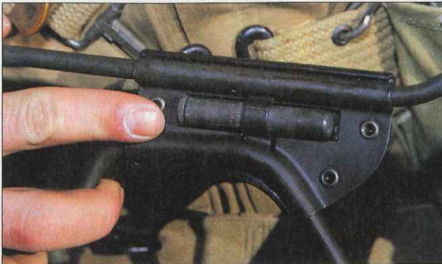
A small metal oil bottle was held in a spring clip behind the M1A1's leather cheekpiece.
