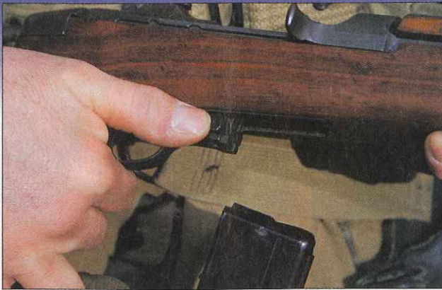
An empty M1 Carbine magazine was dropped by simply pressing in on a release button.
