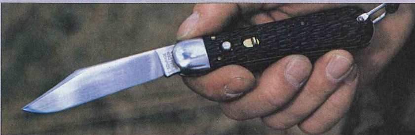
The M2 switchblade knife, manufactured by Schrade, was carried in the jump jacket and was intended to be used for cutting shroud lines should one become entangled.
