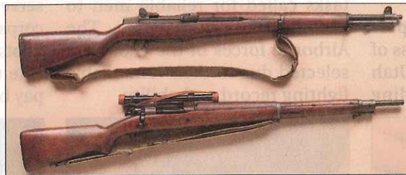
The semiautomatic M1 Garand (top) was the principal U.S. infantry arm during World War II. It was chambered for the .30-06 service cartridge and held eight rounds. Some Paratroopers were issued with M1903A4 sniper rifles (bottom). These five-shot bolt-action repeaters were variants of the O3A3, which, in turn, were simplified versions of the M1903 Springfield. They were topped with 4X Lyman or Weaver scopes.
