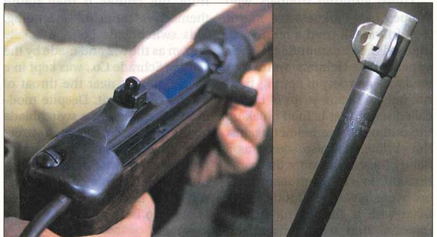
The sights on the M1 Carbine involved a simple flip rear graduated to 150 and 300 yards. The front sight was a simple notch, set within a pair of protective "wings." Notice the "Inland" markings. Inland was the only manufacturer of the M1A1s.
