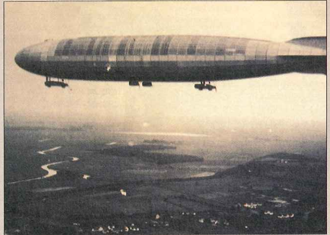
Zeppelins, on average, were 650 feet in length, 2 million cubic feet in volume, 80 feet in diameter and had 16 gas cells. The five 1,200 horsepower Maybach engines could propel the behemoths along at 65 mph.
