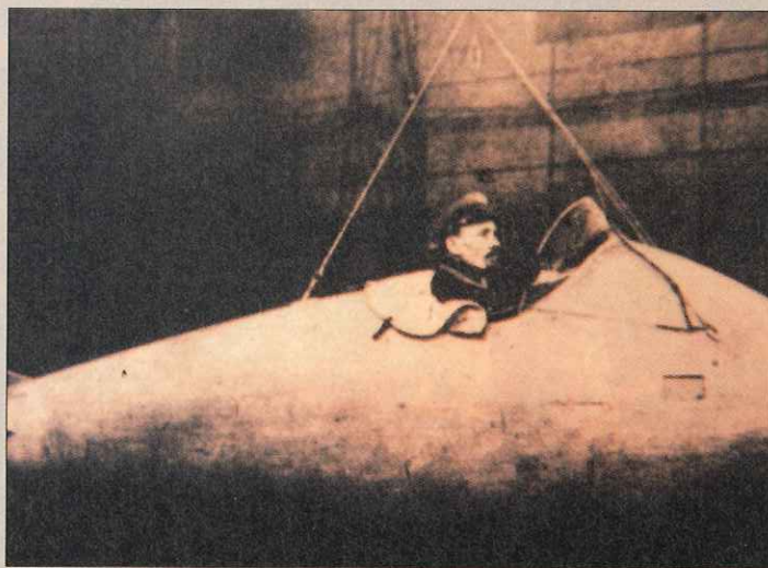
At first, cloudless, moonless nights were thought to be the best for airship raids. With the development of an observation gondola, cloud cover provided a useful screen against the probing searchlights of anti aircraft batteries.
