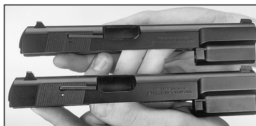
The .40 cal. version has an extra recoil lug on its barrel and a matching recess inside a slide that is 1/4" longer than the original 9 mm Parabellum pistol's.
