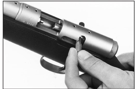
Pushing the cocking handle forward from the cocked position until it is held in place by the cutout on the receiver locks the hammer as a second safety.
