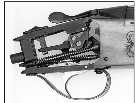
Coil springs power the Condor's hammers, which are controlled by sears that are suspended from the top strap. The manual safety disengages trigger from the connector.
