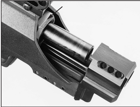
When the Quik-Comp is properly installed on the Scope Mount, the lip at the rear of the comp's top surface matches up with the slide bevel (arrow).
