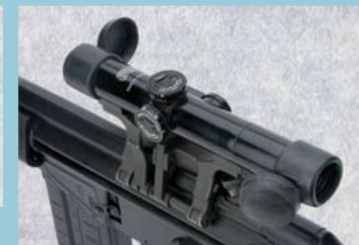
For accuracy testing, we attached an original HK claw mount and Hensoldt 4X scope provided by Century International Arms, Inc.
