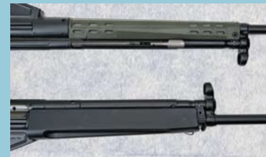
The PTR-91KP (bottom) differs from a standard PTR-91 (top) in that the entire front end of the rifle has been shortened to make the rifle both lighter and more compact.
