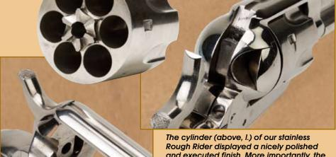
and executed finish. More importantly, the cylinder notches were sharply defined and evenly cut for both hand and locking-bolt engagement.
