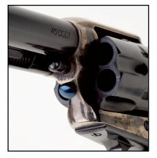
The Cimarron Buntline loads through a loading gate on the right side of its case-colored frame (above). It comes with two cylinder screws, the knurled style (above, r.) and the more traditional slotted style.
