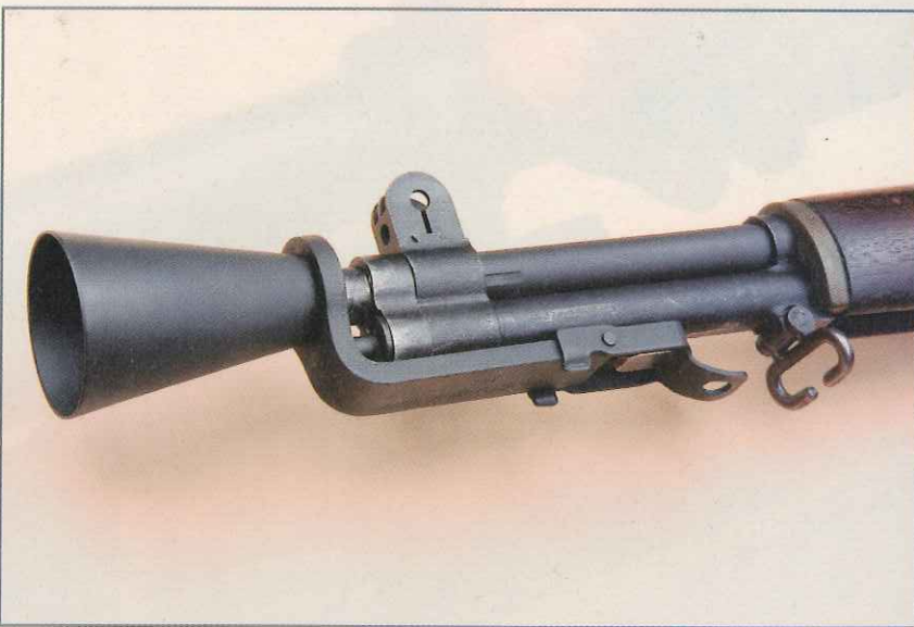
The detachable M2 flash-hider slipped over the rifle's muzzle and was secured by a clip on the bayonet lug.
