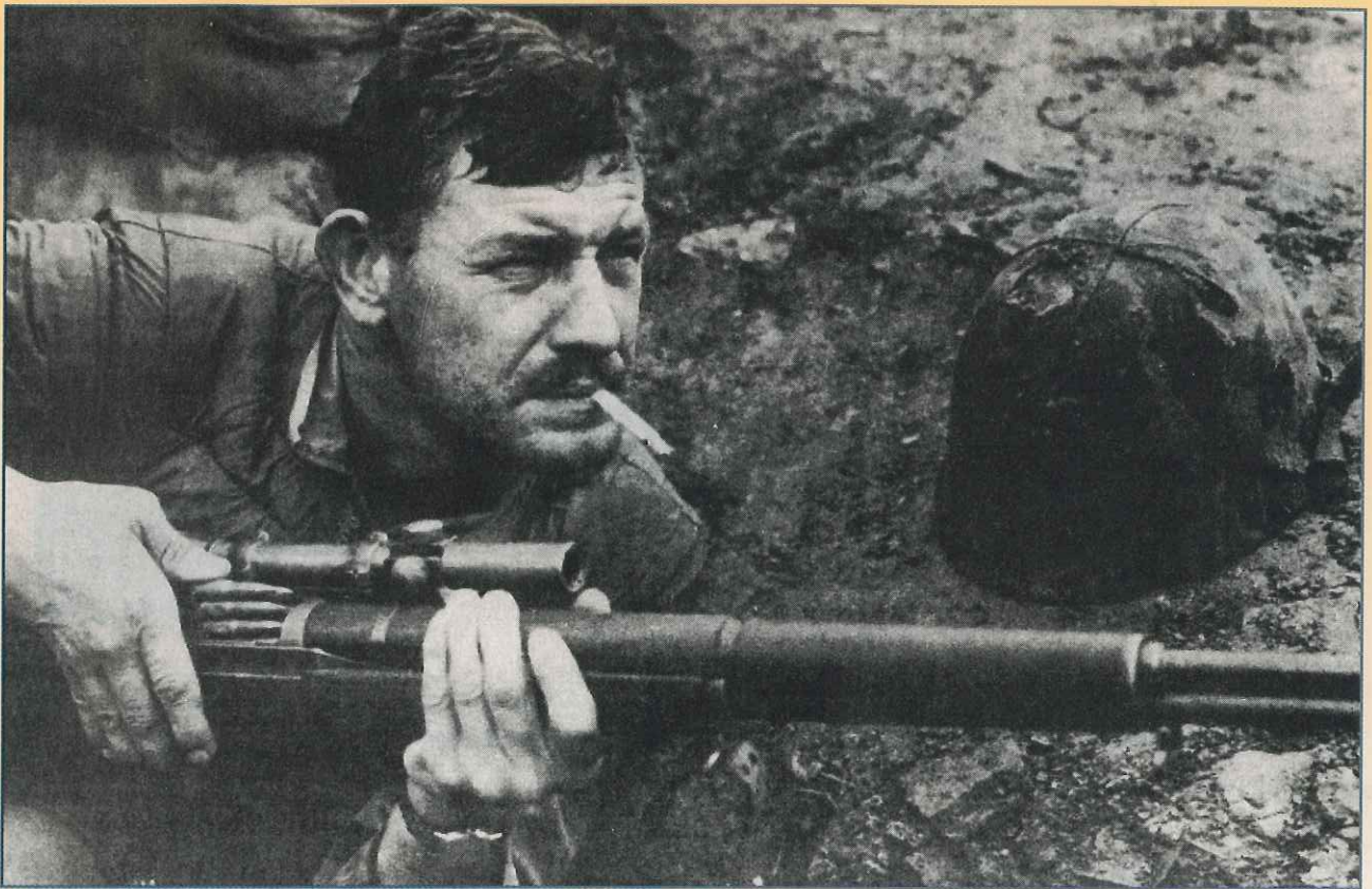
This Marine in Korea loads his M1C rifle with an eight-round clip. The offset mounting setup allowed for easy charging and ejection of the spent clip.
