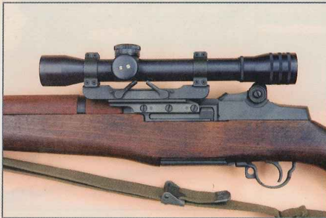
Marine Corps MC 1952 M1C sniper rifles are not as commonly seen as M1Cs and M1Ds. They used a special MC-1 mount and 4X MC-1 Kollmorgen scope.
