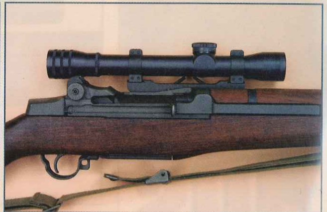
Marine Corps MC 1952 M1C sniper rifles are not as commonly seen as M1Cs and M1Ds. They used a special MC-1 mount and 4X MC-1 Kollmorgen scope.
