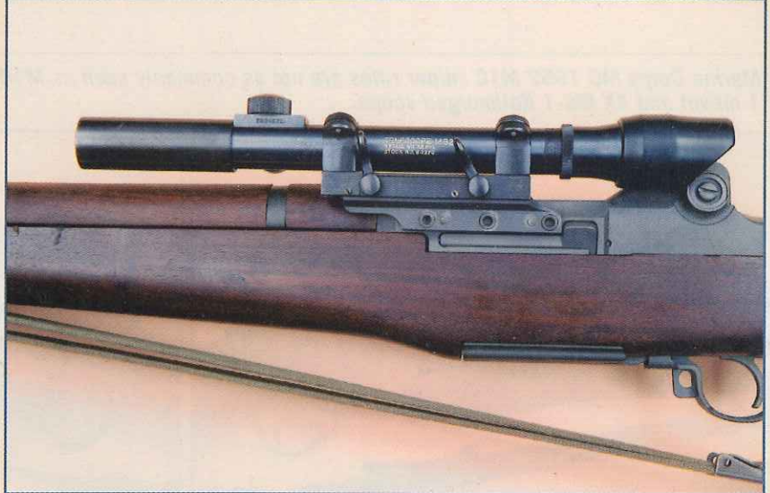
The M1C featured a 2½X M82 Lyman Alaskan scope, secured to the rifle by a Griffin & Howe mounting system.
