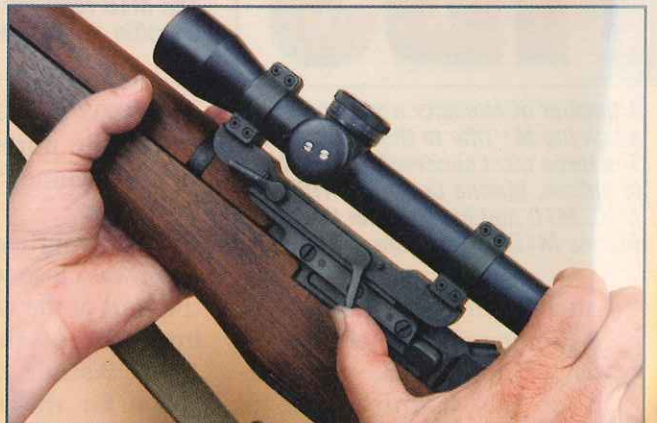
The 4X USMC Kollmorgen scope featured an aluminum tube. It was a variant of the civilian Stith Bear Cub and was painted black.
