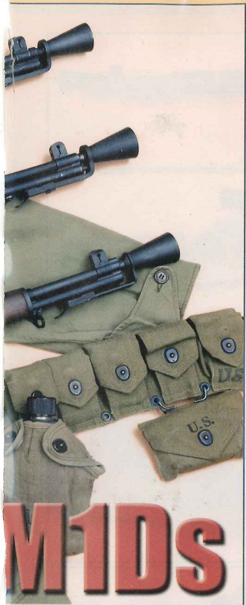
The M1C featured a 2½X M82 Lyman Alaskan scope, secured to the rifle by a Griffin & Howe mounting system.
