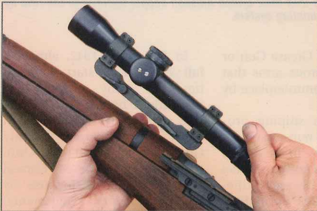
The 4X USMC Kollmorgen scope featured an aluminum tube. It was a variant of the civilian Stith Bear Cub and was painted black.
