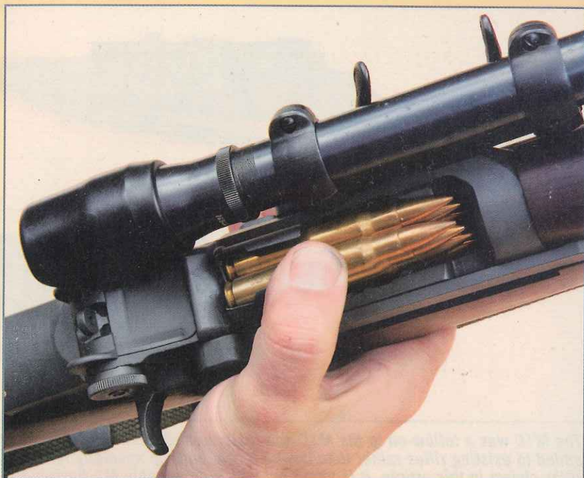
Because of the Garand's unique charging system, it was necessary to offset scopes in order to load the en-bloc clip.
