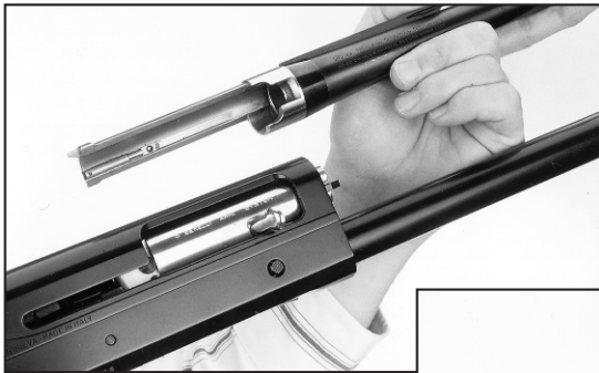
The Super 90 has an aluminum receiver with a chrome-lined barrel (top). The rotating bolt (r.) locks into the barrel extension and is unlocked by the carrier movement.
