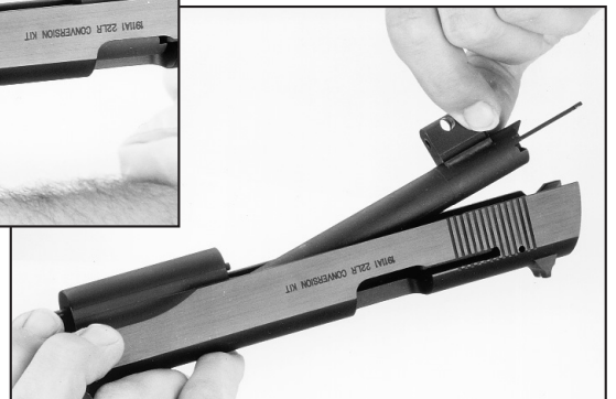
Disassembly is easy with the slide removed from the frame. Retract the recoil spring and its guide rod (top). While holding the unit tightly, lift the barrel up and out of the slide.
