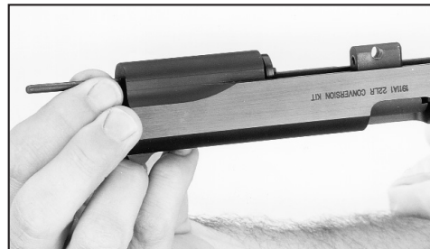
Disassembly is easy with the slide removed from the frame. Retract the recoil spring and its guide rod (top). While holding the unit tightly, lift the barrel up and out of the slide.
