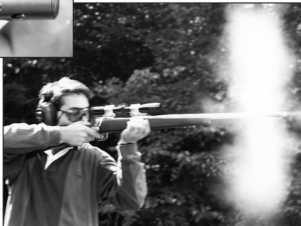
Rotating the outer sleeve of the brake closes off its 33 holes. In firing (r.), the brake proved to be very effective in limiting the felt recoil.
