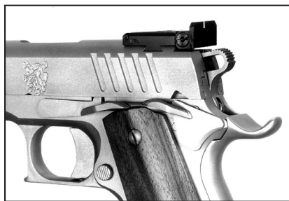
Rear view showing the LPA adjustable sight, wide, angled slide serrations, beavertail grip safety, skeletonized hammer, lightweight aluminum trigger, and extended thumb safety and slide release.
