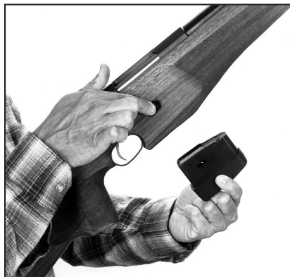
A serrated button in the right side of the stock is depressed to release the single-column five-round magazine. Magazine release can also be performed with the left hand reaching around under the stock.
