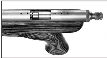
The leg can be used to support the Hawkeye during loading (above l.). The drilled and tapped holes in the Hawkeye's receiver (r.) allow the mounting of a telescopic sight or the supplied iron sights.
