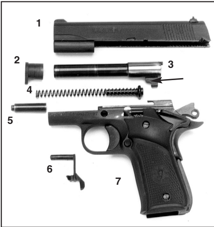
The Micromax field-stripped, showing its (1) slide, (2) barrel bushing, (3) barrel, (4) recoil spring and guide, (5) spring plug, (6) slide stop and (7) frame. The semicircular cut in the barrel underlug (arrow) engages the slide stop pin and positions the barrel.
