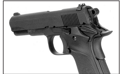
Seen here are the Llama's beavertail grip safety, thumb safety, extended slide stop, Commander-style hammer, plastic thumb-rest stocks and fixed three-dot sights.
