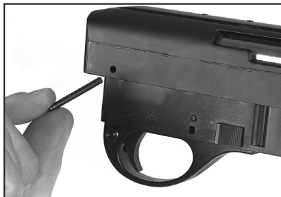
The 597's magazine housing and trigger assembly are one plastic piece separated by a solid web of plastic. It is fastened to the gun's steel receiver by an assembly pin.
