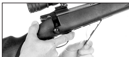
The integral magazine has a hinged steel floorplate that is opened by depressing a latch on the front of the 1500's trigger guard.
