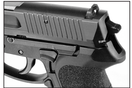
The Sig Pro has twelve angular grasping grooves on each side of the slide. A decocker and slide release are on the left.
