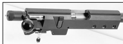
The new KK200's turn-bolt, single-shot action features a flat bottom, carbon steel receiver. The barrel is clamped in place by three socket-head bolts on the right side.
