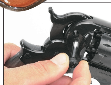
A throughbolt secures the hinged, two-piece frame at the top of the standing breech. It is easily removed for cleaning.
