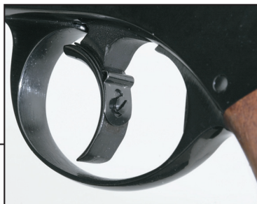
The front "trigger" is the cocking lever. It functions as the trigger when the Starr is in the double-action mode. The trigger proper is the small tab in the rear of the trigger guard.
