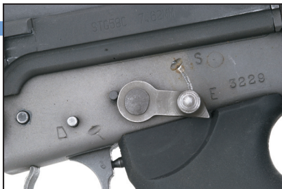
The STG58 has a two-position safety lever on the left side of the lower receiver. In the safe position the pointer will be in the upper right position marked "S."
