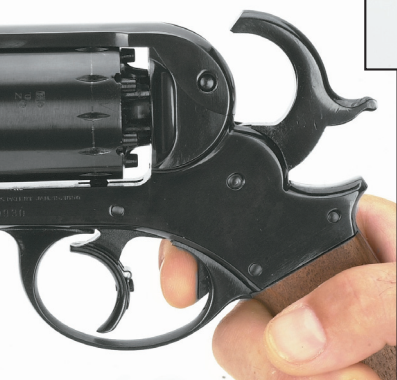
The front "trigger" is the cocking lever. It functions as the trigger when the Starr is in the double-action mode. The trigger proper is the small tab in the rear of the trigger guard.
