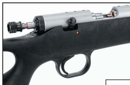
Behind the breech plug, the top half of the barrel/receiver is milled out to form a priming port. The port is not very large, and an in-line capper will be necessary for most shooters.
