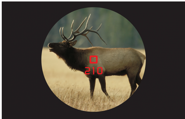
A precise internal clock times the round trip of a series of laser pulses, then converts that data into distance displayed as a highly visible LCD readout inside the rangefinder.
