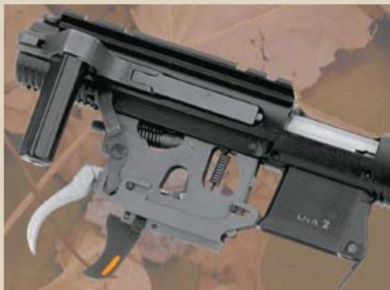
The sample rifle's trigger broke at 2¼ lbs., which contributed to the rifle's accuracy. The safety is actually in the front of the trigger guard, much like an M1 Garand.
