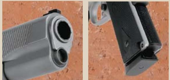
Smith & Wesson uses several recognizable aftermarket parts in its 1911 pistol. An example of that is the machined aluminum mainpring housing (r.), which is used instead of an equivalent plastic part seen on many other pistols. The stainless steel barrel has a slightly oversize area near the muzzle to promote a better barrel to bushing fit (l.). The fit of the bushing to the slide does not necessitate a wrench for turning, but is not overly loose, either.
