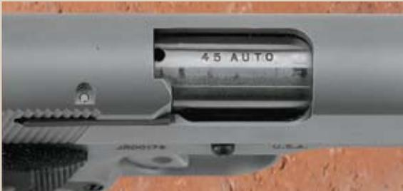
The barrel is a standard M1911 style with a small "U"-shaped cutout on the hood to allow the shooter to view whether there is a cartridge in the chamber or not.
