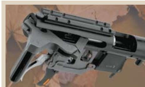
The Basic's action has two jointed arms with three pivot points—one on the rear of the bolt, one on the rear receiver bridge and one linking the two arms together (arrows above). Here, the action is unlocked and the arms are pivoted.
