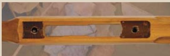
To enhance accuracy, the Biathlon Basic action is bedded under both the receiver ring and the action's rear.
