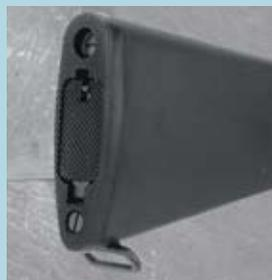
The Rock River Arms Varmint's A2-style buttstock has trap-door access to a storage compartment that could be used to add weight and change the gun's center of balance. A two-stage match trigger (r.) breaks cleanly to aid accuracy.
