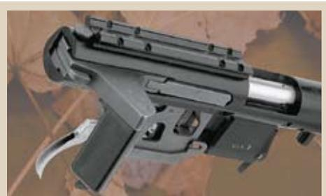
Pressing the operating handle forward advances the bolt, stripping a cartridge from the magazine and chambering it. As the bolt travels forward, the center pivot moves inward, causing the arms and pivots to line up and lock the bolt.
