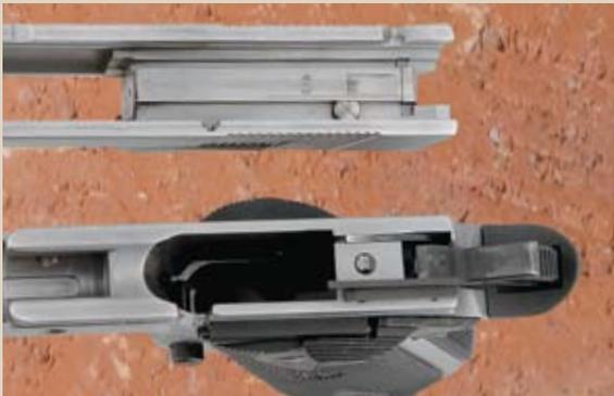
S&W uses a variant of the Swartz firing pin safety that has a crescent-shaped lifter located beside the hammer (1) and is held in place by the hammer pin. When the grip safety is depressed, the firing pin lock (2) is lifted.
