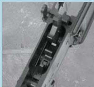
patible Weaver-style optical mount runs the length of Rock River's EOP upper receiver. Additionally, the rear of the receiver bridge is dished to accommodate the large eyepieces common to high magnification varmint scopes.
