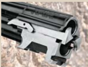
The barrels employ the monobloc principle. A tapered notch (arrow) is engaged by locking bolt.
