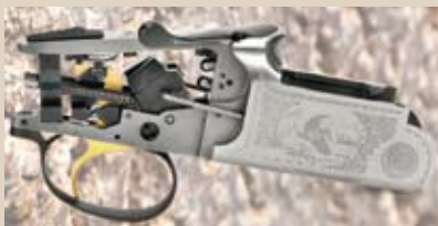
The barrels employ the monobloc principle. A tapered notch (arrow) is engaged by locking bolt.
