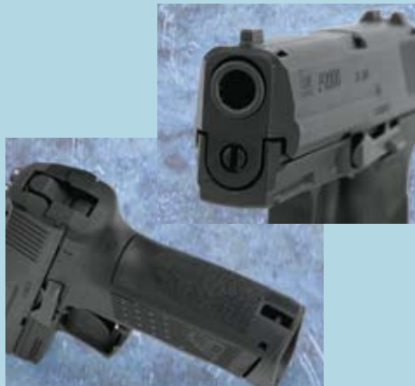
The slide's front face is scalloped (top) to ease holster insertion. Each gun comes with three backstrap inserts that can be changed out by driving out the roll pin at the bottom rear.
