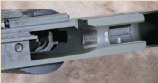
The CQB's polished feed ramp (arrow) is one of many touches that adds to the pistol's reliability and is another sign of Wilson's attention to detail.
