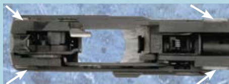
Steel inserts (arrows) are molded in on each side of the fiber-reinforced polymer frame for slide-bearing surfaces.
