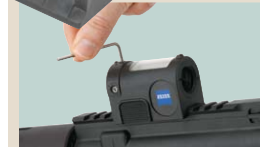
The Z-Point is designed to easily snap on and off any standard Picatinny rail by way of a single, spring-loaded, push-button clamp that "rocks" over the rail.
