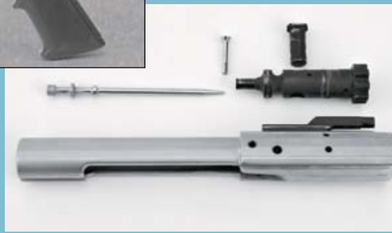
The Panther 308's bolt carrier (r.) is somewhat different from those of other .308 AR-based rifles. The carrier is machined from Carpenter 158 chrome molybdenum steel and hard chrome-plated. The bolt itself is dimensionally similar to those of other .308 AR-10-type rifles.
