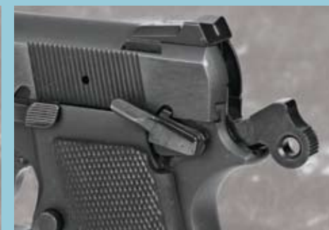
XS sights (above, l.) are a welcome addition, though we'd prefer the tritium version. The cost, though, would substantially raise the HP's price. The thumb safety (center) is well sized for
