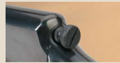
Like the original Winchester, Taurus' replica is a take-down model. Turning out the knurled knob at the rear of the receiver allows the rifle to separate for transport or cleaning.
