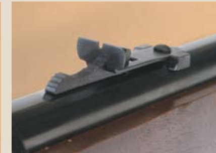
Although the front sight post is fixed, the rear blade is step-adjustable for elevation and drift-adjustable for windage.
