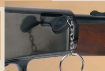
Safety features include a cross-bolt safety button at the rear of the trigger guard and the Taurus Security System lock on the bolt. Turning out the lock with the supplied key locks the bolt closed and prevents movement of the firing pin.
