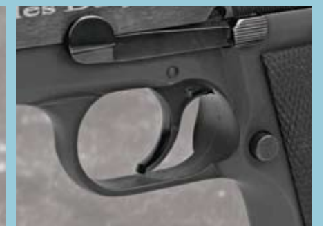
easy manipulation, while the rowel hammer reduces bite. The trigger (r.) is gritty and heavy, however, the improved extended slide release lever above it is a nice added feature.
