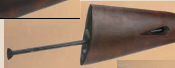
The Taurus 63's fixed tubular magazine is housed in the stock. The follower can be removed through a hole in the buttplate and rounds may be loaded through a port in the side of the stock.
