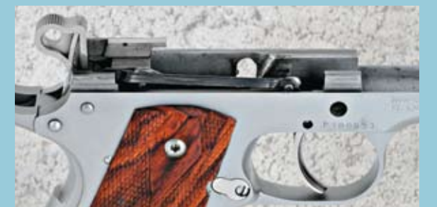
The trigger bar of the LDA mechanism occupies space usually taken up by the right frame rail. LDA pistols are made of steel to assure strength in the abbreviated rail.
