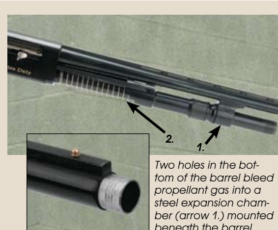
Expanding gas pushes the piston, spacer and action rod assembly rearward against the recoil spring (arrow 2.). Unlike most 28-ga. autoloaders, the Daly comes with interchangeable choke tubes (1.).
