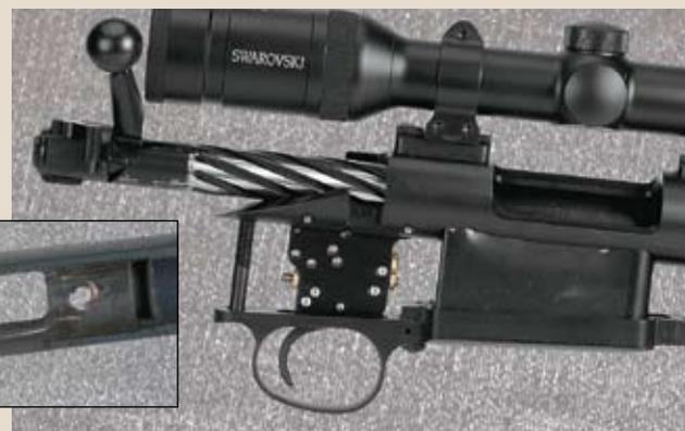
Ed Brown's Model 702 action has a 1.36"-diameter cylindrical receiver of 4140 chrome-moly steel that is heat-treated before it is machined from bar stock.
