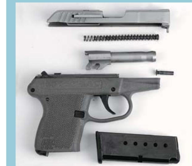
The P-3AT strips to its major components with removal of a single pin. There's just the slide, nested recoil springs, guide rod, barrel, assembly pin, frame and magazine.
