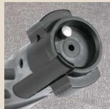
The two-lug bolt is of 8620 steel and has a 0.702" body diameter, a 0.98" diameter across the lug circle. The extractor is a .249"-wide, AR-15-style unit, while ejection is via a spring-loaded plunger in the bolt face.
