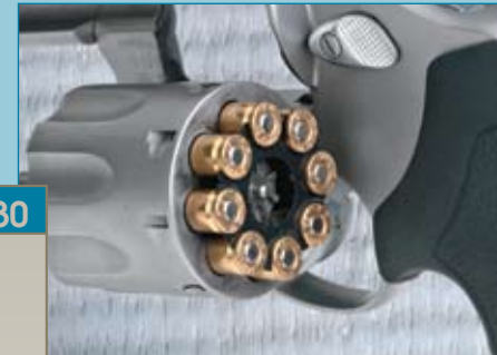
Cylinder capacity for the gun is eight .30 Carbine cartridges (r.) that are mounted in sheet steel Stellar Clips.
