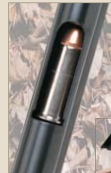
The .44 Mag. Big Boy loads from the end of the magazine tube in the manner of many .22 rimfires. This was found to be easy and speedy.
