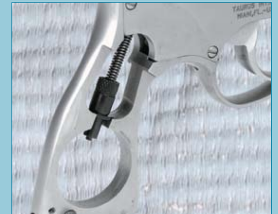
The tension on the mainspring (which affects trigger pull) is hand-adjustable via a knurled retaining nut inside the grip frame.
