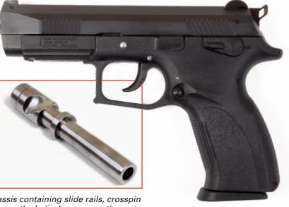
The polymer frame houses the steel chassis containing slide rails, crosspin and trigger group (l.). The crosspin engages the helical groove on the carbon-nitrided steel barrel (r.) during rotary-locked, short-recoil operation. Optimal ergonomics provide a comfortable, low-profile grip (above, r.).
